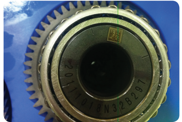
A low-contrast 2-D Data Matrix code on a Kia Motors transmission part. The Cognex 2DMax+ code reading algorithm can read virtually any barcode regardless of the damage or the surface it is marked on.
