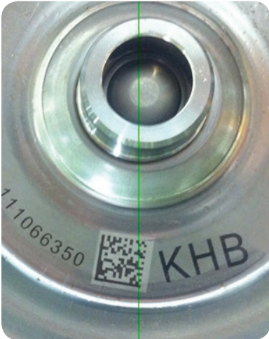
A 2-D Data Matrix code on a Kia Motors car transmission part. DataMan barcode readers are optimized with a patented algorithm which helps users achieve the highest read rates (99.9%) in the toughest Direct Part Mark (DPM) and label-based ID applications.
